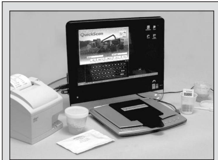
Here's the package of technology that comprises the GMO-testing "Quick Scan 131" system from Envirologix. Snowville Creamery has recently purchased and started using this system to test for GMO materials in the feeds of its ten dairy producers. More information about Envirologix may be found at the firm's Web site: <http://envirologix.com/>
